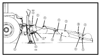
Figure 8A - Lubrication Points for Model 965H
